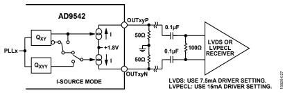
Figure 31. LVDS-Compatible Output Swing, AC-Coupled (V p-p  $\approx$  375 mV per Section for I = 15 mA
