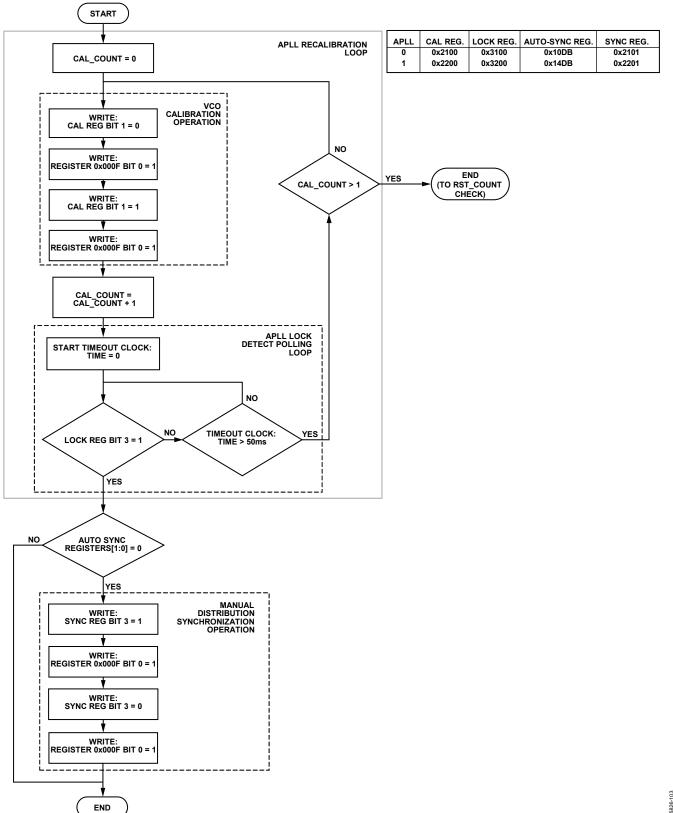
Figure 45. Analog PLL Initialization Subprocess
