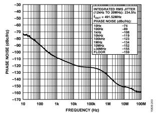
Figure 5. Absolute Phase Noise (PLL0, Configuration 3, HCSL Mode,  $f_{\rm REF}=1$  Hz,  $f_{\rm OUT}=491.52$  MHz,  $f_{\rm COMP}=19.2$  MHz TCXO,  $f_{\rm SYS}=52$  MHz Crystal, 50 MHz DPLL BW)
