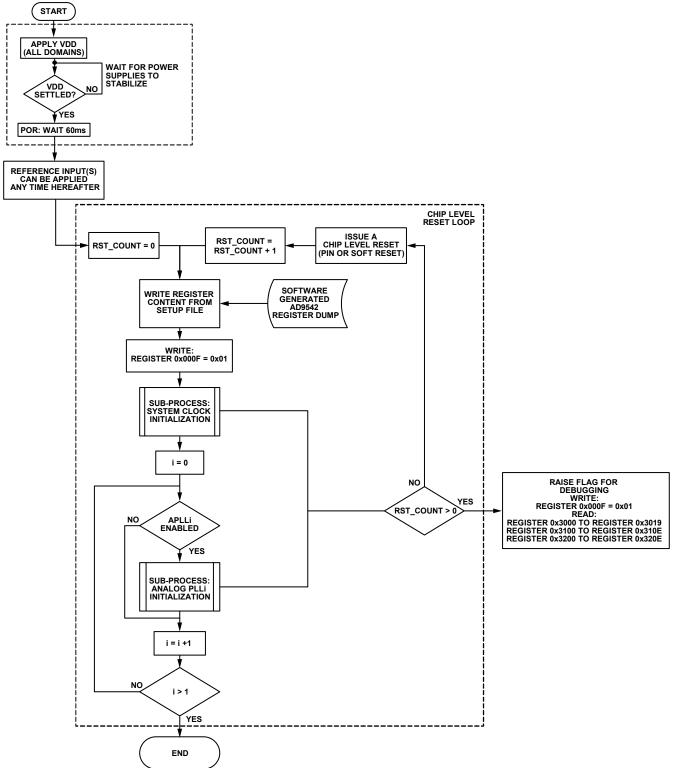
Figure 43. Programming Sequence Loop
