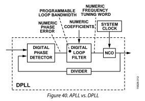
The DPLLs in the AD9542 have a digital TDC-based phase detector and a digital loop filter with programmable bandwidth. The digital loop filter output yields a digital FTW (instead of a dc voltage, as in the case of an analog PLL) that produces a corresponding NCO output frequency.
