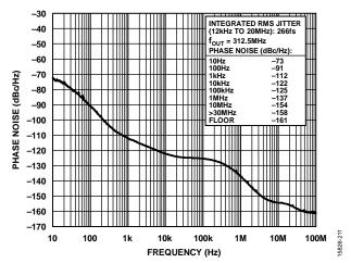
Figure 13. Absolute Phase Noise (PLL1, Configuration 5, HCSL Mode,  $f_{\rm REF}$  = 25 MHz,  $f_{\rm OUT}$  = 312.5 MHz,  $f_{\rm SYS}$  = 52 MHz Crystal, 50 Hz DPLL BW, Phase Buildout Mode)
