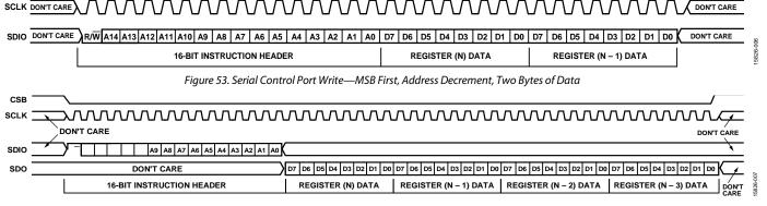
Figure 54. Serial Control Port Read—MSB First, Address Decrement, Four Bytes of Data
