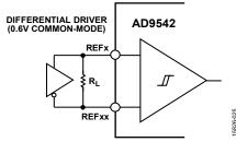
Figure 30. Differential DC-Coupled Mode
