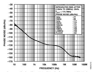
Figure 14. Absolute Phase Noise (PLL1, Configuration 6, HCSL Mode,  $f_{\rm REF} = 155.52$  MHz,  $f_{\rm OUT} = 174.7$  MHz,  $f_{\rm SYS} = 52$  MHz Crystal, 50 Hz DPLL BW, Phase Buildout Mode)
