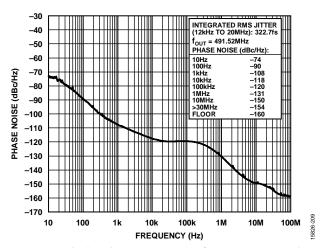
Figure 11. Absolute Phase Noise (PLL1, Configuration 3, HCSL Mode,  $f_{\rm REF}=1$  Hz,  $f_{\rm OUT}=491.52$  MHz,  $f_{\rm COMP}=19.2$  MHz TCXO,  $f_{\rm SYS}=52$  MHz Crystal, 50 MHz DPLL BW)
