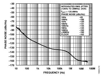
Figure 12. Absolute Phase Noise (PLL1, Configuration 4, HCSL Mode,  $f_{REF} = 125$  MHz,  $f_{OUT} = 125$  MHz,  $f_{COMP} = 19.2$  MHz TCXO,  $f_{SYS} = 52$  MHz Crystal, 0.1 Hz DPLL BW, Phase Buildout Mode)
