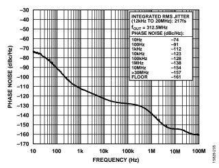
Figure 7. Absolute Phase Noise (PLL0, Configuration 5, HCSL Mode,  $f_{\rm REF}$  = 25 MHz,  $f_{\rm OUT}$  = 312.5 MHz,  $f_{\rm SYS}$  = 52 MHz Crystal, 50 Hz DPLL BW, Phase Buildout Mode)
