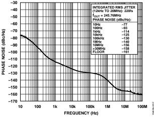
Figure 4. Absolute Phase Noise (PLL0, Configuration 2, HCSL Mode,  $f_{\rm REF}$  = 30.72 MHz,  $f_{\rm OUT}$  = 245.76 MHz,  $f_{\rm SYS}$  = 52 MHz Crystal, 50 Hz DPLL BW)
