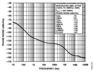
Figure 10. Absolute Phase Noise (PLL1, Configuration 2, HCSL Mode,  $f_{\rm REF}$  = 30.72 MHz,  $f_{\rm OUT}$  = 245.76 MHz,  $f_{\rm SYS}$  = 52 MHz Crystal, 50 Hz DPLL BW)
