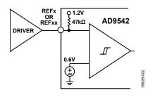
Figure 27. Single-Ended Internal Pull-Up Mode
