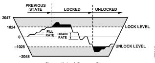
Figure 49. Lock Detector Diagram
