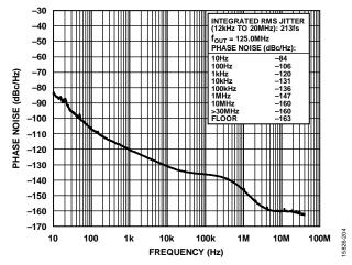
Figure 6. Absolute Phase Noise (PLL0, Configuration 4, HCSL Mode,  $f_{\rm REF}$  = 125 MHz,  $f_{\rm OUT}$  = 125.0 MHz,  $f_{\rm COMP}$  = 19.2 MHz TCXO,  $f_{\rm SYS}$  = 52 MHz Crystal, 0.1 Hz DPLL BW, Phase Buildout Mode)
