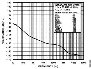
Figure 8. Absolute Phase Noise (PLL0, Configuration 6, HCSL Mode,  $f_{\rm REF}$  = 155.52 MHz,  $f_{\rm OUT}$  = 174.7 MHz,  $f_{\rm SYS}$  = 52 MHz Crystal, 50 Hz DPLL BW, Phase Buildout Mode)
