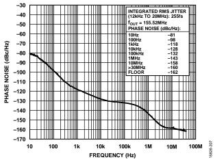
Figure 9. Absolute Phase Noise (PLL1, Configuration 1, HCSL Mode,  $f_{\rm REF} = 38.88~{\rm MHz}$ ,  $f_{\rm OUT} = 155.52~{\rm MHz}$ ,  $f_{\rm SYS} = 52~{\rm MHz}$  Crystal, 50 Hz DPLL BW)
