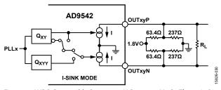
Figure 35. LVDS-Compatible Output, 1.2 V Common-Mode, Thevenin Bias Network (I=7.5 mA; 15 mA With Extra 100  $\Omega$  Termination,  $R_L$ )
