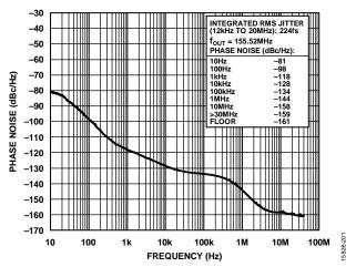
Figure 3. Absolute Phase Noise (PLL0, Configuration 1, HCSL Mode,  $f_{\rm REF}=38.88~{\rm MHz}$ ,  $f_{\rm OUT}=155.52~{\rm MHz}$ ,  $f_{\rm SYS}=52~{\rm MHz}$  Crystal, 50 Hz DPLL BW)
