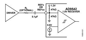
Figure 26. Single-Ended AC-Coupled Mode
