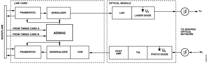
Figure 41. Optical Line Card Example
