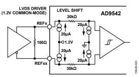
Figure 28. Differential LVDS Input Mode
