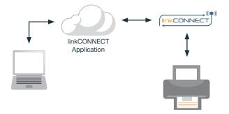
Siretta linkCONNECT solutions are used in remote printing applications to enable standard Windows / Linux printer drivers to print directly to remote devices. The printer driver TCP/IP port can be used to connect directly to the linkCONNECT solution and allow direct printing in the field with no user configuration or setup required.
