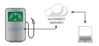
Siretta linkCONNECT solutions are used in pump automation and distribution control system projects where authorisation to distribute fuel / oil / electricity is required via credit card payment or validated company credit account. The linkCONNECT solution provides a point to point link to the distribution point and provides a real time device status which can be used to authorise payments and initiate delivery of the service.
