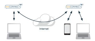
Siretta linkCONNECT solutions are used in applications to link end devices, end systems and end components together. Once setup the linkCONNECT solution automates the connection procedure and removes the need to understand or know the underlying connection information. This enables linkCONNECT devices to be configured once before shipping and then the end user simply plugs in the device and they are immediately ready to connect with no setup required.
