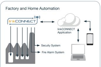
Siretta linkCONNECT solutions can be used in factory automation projects to link the factory to the factory manager or service manager. The information can be displayed on a mobile application on a smart phone or more detailed statistics can be presented through a standard PC application over a web browser.
