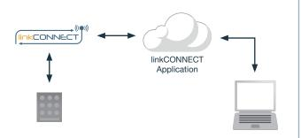
Siretta linkCONNECT solutions are used in remote door entry applications to authenticate users via either a simple pin code entry mechanism or a more advanced system such as fingerprint recognition or Bluetooth phone authentication. Once user is authenticated the system is able to securely grant access to building premises, warehouses, garages etc without the need for a manual key exchange or a lock and key entry.
