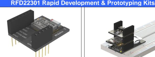
RFD22102 DIP version of RFD22301 for prototyping
