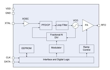
Figure 11. RFM119W/RFM119SW Functional Block Diagram
