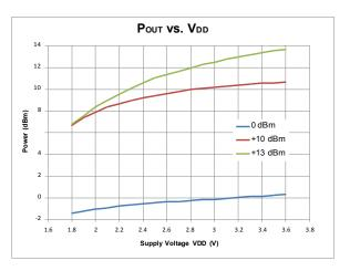
Figure 8. Output Power vs. Supply Voltages, F<sub>RF</sub> = 433.92 MHz
