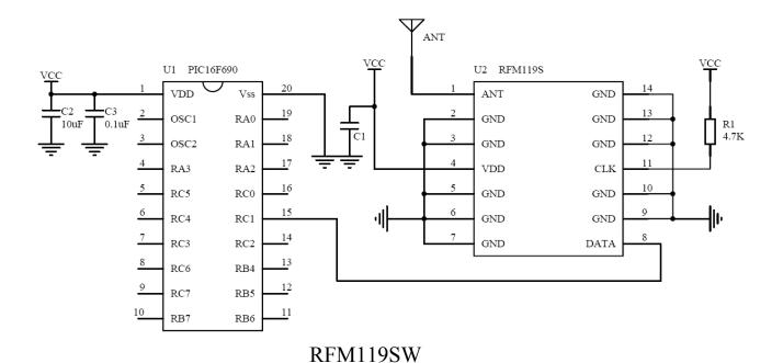
Figure 9: Typical Application Schematic
