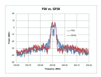
Figure 6. FSK/GFSK Spectrum, SR = 9.6 ksps,  $F_{DEV}$  = 15 kHz
