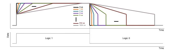
Figure 13. PA Ramping Time
