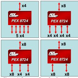
Figure 1. Common Port Configurations
