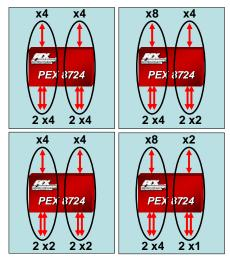
Figure 2. Multi-Host Port Configurations
