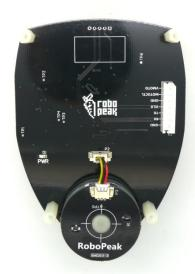
RPLIDAR development kit contains standard RPLIDAR unit (A1M1-R1). The RPLIDAR embedded logic IO drivable (3.3V) motor controller which can be used to configure scan frequency by tuning motor speed. Developer also can choose to turn off motor for power saving purpose.
