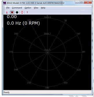
The firmware/hardware version and serial number of the RPLIDAR will show in the title line of the GUI. The supported commands of RPLIDAR are showed in the tool bar. The descriptions are listed in the bellow table.
