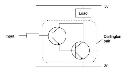
The current gain varies for different transistor and can be looked up in the datasheet for the device. Typically, it may be 100. This would mean that the current available to drive the load would be 100 times larger than the input to the transistor.
