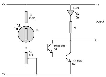
The circuit operation is very simple. When the input to the transistor Q1, which is fed from the connecting point of R1 and R2, is greater than 1.4V, the output is turned on. The voltage at the join of R1 and R2 is determined by the ratio of the two resistors. This is known as potential divider.
