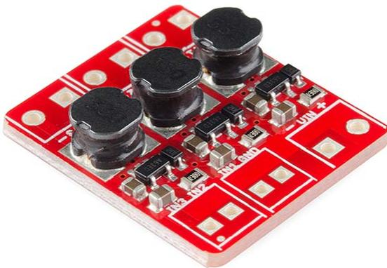
Developed in collaboration with Ethan Zonca of protofusion, the PicoBuck is a small-size triple-output constant current LED driver. By default, each channel is driven at 350mA; that current can be reduced by either presenting an analog voltage or a PWM signal to the board.
