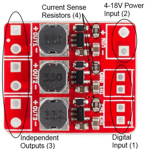
Three signal inputs (1) are provided for dimming control. A separate ground pin is provided to reference against the controlling module for accuracy.
