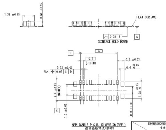
Note 1) Dimension 3.9±0.05 is recommended in case repair is needed.
