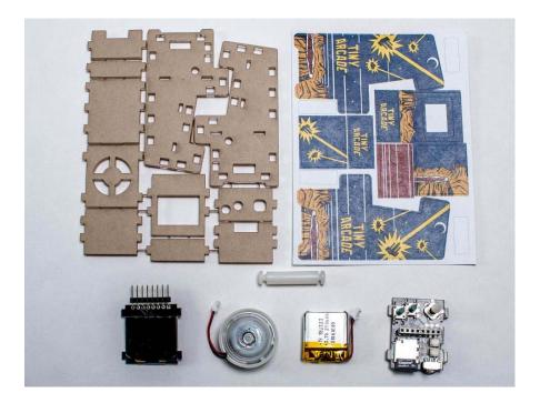
The Tiny Arcade is simple to put together - there is no soldering needed, or any special tools. The circuit boards fit together and the acrylic cases assemble like a jigsaw puzzle with no glue needed. It only takes about **10 minutes** to assemble a Tiny Arcade. Check out the assembly instructions.
