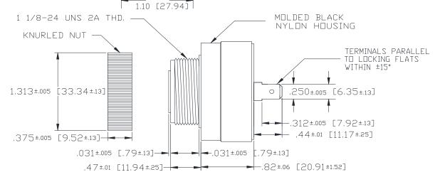
MOUNTING: REMOVE BLACK PLASTIC NUT AND INSERT THREADED FRONT THROUGH 1.25"
