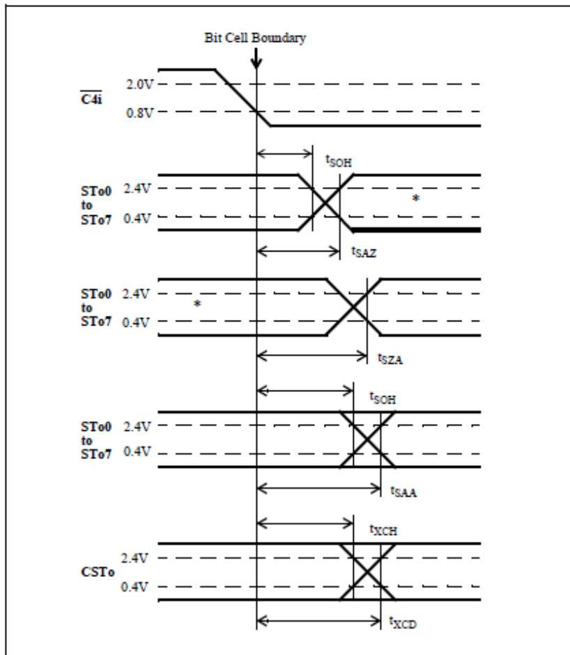
Figure 14 - Serial Outputs and External Control
