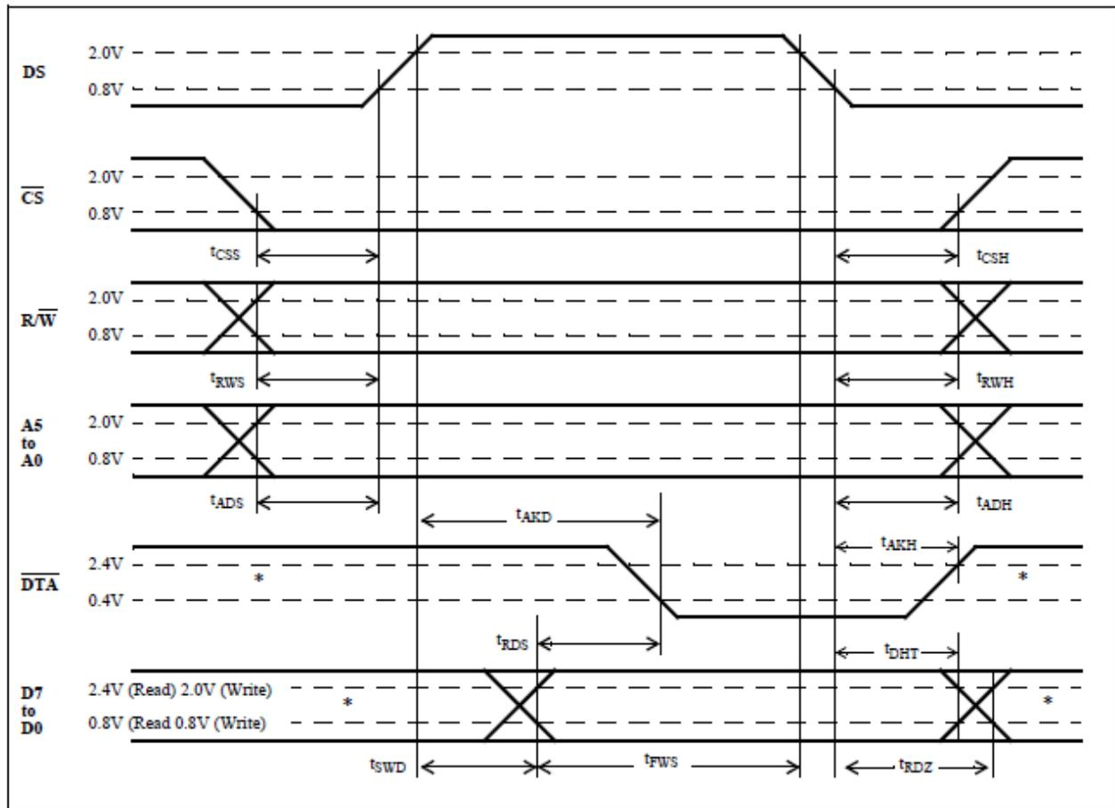
Figure 17 - Processor Bus
