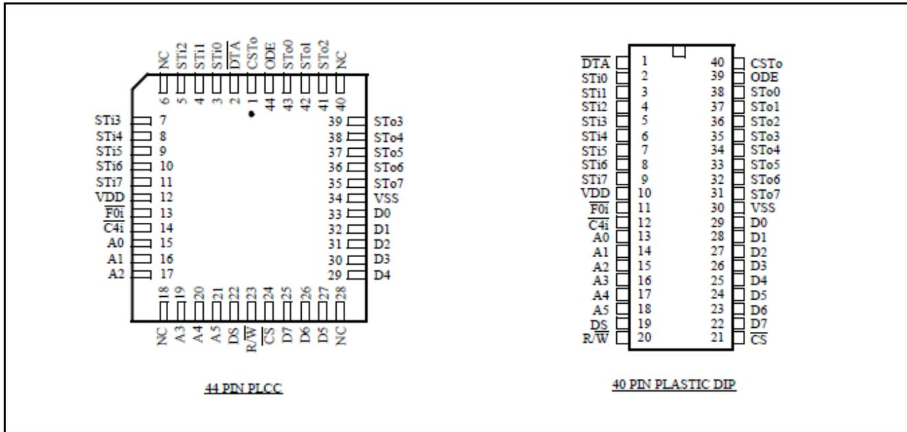
**Figure 2 - Pin Connections**
