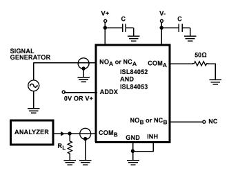
FIGURE 6. CROSSTALK TEST CIRCUIT
