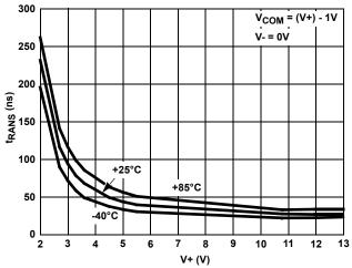
FIGURE 15. ADDRESS TRANS TIME vs SINGLE SUPPLY VOLTAGE
