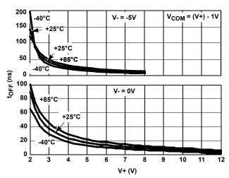
FIGURE 14. INHIBIT TURN-OFF TIME vs SUPPLY VOLTAGE
