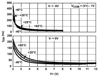
FIGURE 13. INHIBIT TURN-ON TIME vs SUPPLY VOLTAGE
