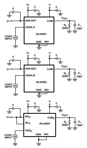
Repeat test for other switches.  $C_L$  includes fixture and stray capacitance.
