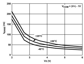
FIGURE 16. ADDRESS TRANS TIME vs DUAL SUPPLY VOLTAGE
