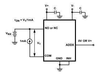
FIGURE 5. ron TEST CIRCUIT
