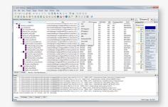
In addition to showing the design hierarchy, important information is available here such as source files used, and both post-synthesis and post-map resources used.
