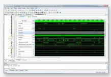
The Reveal Hardware Debugger uses a signal-centric model that allows easy insertion of embedded logic analyzer debug hardware for real-time analysis.
